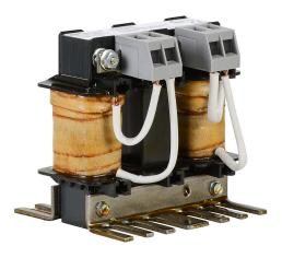
AutomationDirect LR series line reactor, 110 VAC, 1/3hp, 1-phase, 8A, 3% impedance, input side only. For use with multiple AC drives.
