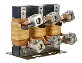
AutomationDirect LR series line reactor, 230 VAC, 100hp, 3-phase, 273A, 3% impedance, input or output side. For use with multiple AC drives.
