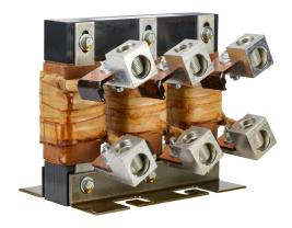
AutomationDirect LR series line reactor, 230 VAC, 75hp, 3-phase, 211A, 3% impedance, input or output side. For use with multiple AC drives.
