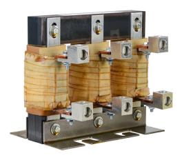
AutomationDirect LR series line reactor, 230 VAC, 60hp, 3-phase, 169A, 3% impedance, input or output side. For use with multiple AC drives.
