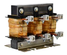
AutomationDirect LR series line reactor, 230 VAC, 30hp, 3-phase, 88A, 3% impedance, input or output side. For use with multiple AC drives.
