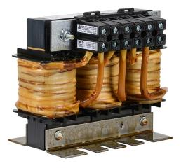
AutomationDirect LR series line reactor, 230 VAC, 25hp, 3-phase, 74.8A, 3% impedance, input or output side. For use with multiple AC drives.
