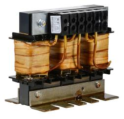
AutomationDirect LR series line reactor, 230 VAC, 10hp, 3-phase, 30.8A, 3% impedance, input or output side. For use with multiple AC drives.
