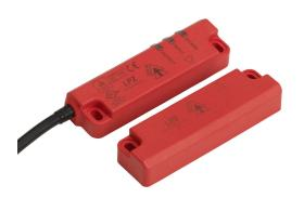
IDEM Z-Range safety switch set, non-contact master coded RFID, (2) OSSD safety output(s), (1) status monitoring output(s), polyester housing, 91 x 26mm, 8-pin M12 quick-disconnect, 9.8in/250mm cable length.
