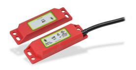
IDEM safety switch set, non-contact magnetic, (2) N.C. safety output(s), (1) N.O. monitoring output(s), plastic housing, 88 x 25mm, pigtail, 6.5ft/2m cable length.
