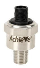
AchieVe pressure transmitter, -14.7 to 30 psig range, +/-1% accuracy, stainless steel sensing element, 4-20 mA analog output, 1/4in male NPT process connection, 9 to 32 VDC operating voltage, 4-pin M12 quick-disconnect.
