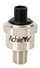
AchieVe pressure transmitter, -14.7 to 30 psig range, +/- 1% accuracy, stainless steel sensing element, 4-20 mA analog output, 1/4in male NPT process connection, 9-32 VDC operating voltage, 4-pin M12 quick-disconnect.
