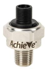
AchieVe pressure transmitter, 0 to 5000 psig range, +/- 1% accuracy, stainless steel sensing element, 4-20 mA analog output, 1/4in male NPT process connection, 9-32 VDC operating voltage, 4-pin M12 quick-disconnect.
