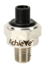
AchieVe pressure transmitter, 0 to 3000 psig range, +/-1% accuracy, stainless steel sensing element, 4-20 mA analog output, 1/4in male NPT process connection, 9 to 32 VDC operating voltage, 4-pin M12 quick-disconnect.
