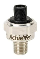
AchieVe pressure transmitter, 0 to 2000 psig range, +/-1% accuracy, stainless steel sensing element, 4-20 mA analog output, 1/4in male NPT process connection, 9 to 32 VDC operating voltage, 4-pin M12 quick-disconnect.
