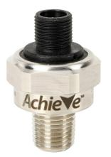
AchieVe pressure transmitter, 0 to 2000 psig range, +/- 1% accuracy, stainless steel sensing element, 4-20 mA analog output, 1/4in male NPT process connection, 9-32 VDC operating voltage, 4-pin M12 quick-disconnect.
