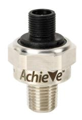
AchieVe pressure transmitter, 0 to 1000 psig range, +/- 1% accuracy, stainless steel sensing element, 4-20 mA analog output, 1/4in male NPT process connection, 9-32 VDC operating voltage, 4-pin M12 quick-disconnect.
