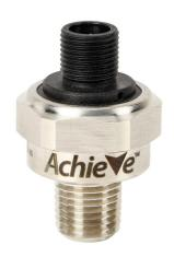
AchieVe pressure transmitter, 0 to 500 psig range, +/-1% accuracy, stainless steel sensing element, 4-20 mA analog output, 1/4in male NPT process connection, 9 to 32 VDC operating voltage, 4-pin M12 quick-disconnect.
