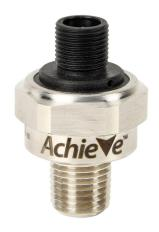
AchieVe pressure transmitter, 0 to 500 psig range, +/- 1% accuracy, stainless steel sensing element, 4-20 mA analog output, 1/4in male NPT process connection, 9-32 VDC operating voltage, 4-pin M12 quick-disconnect.
