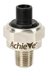
AchieVe pressure transmitter, 0 to 300 psig range, +/- 1% accuracy, stainless steel sensing element, 4-20 mA analog output, 1/4in male NPT process connection, 9-32 VDC operating voltage, 4-pin M12 quick-disconnect.
