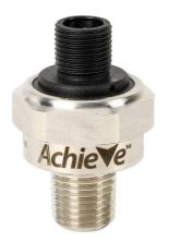
AchieVe pressure transmitter, 0 to 200 psig range, +/- 1% accuracy, stainless steel sensing element, 4-20 mA analog output, 1/4in male NPT process connection, 9-32 VDC operating voltage, 4-pin M12 quick-disconnect.
