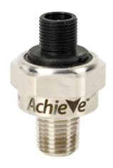
AchieVe pressure transmitter, 0 to 100 psig range, +/-1% accuracy, stainless steel sensing element, 4-20 mA analog output, 1/4in male NPT process connection, 9 to 32 VDC operating voltage, 4-pin M12 quick-disconnect.
