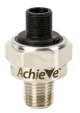
AchieVe pressure transmitter, 0 to 100 psig range, +/- 1% accuracy, stainless steel sensing element, 4-20 mA analog output, 1/4in male NPT process connection, 9-32 VDC operating voltage, 4-pin M12 quick-disconnect.
