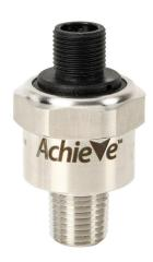
AchieVe pressure transmitter, 0 to 60 psig range, +/-1% accuracy, stainless steel sensing element, 4-20 mA analog output, 1/4in male NPT process connection, 9 to 32 VDC operating voltage, 4-pin M12 quick-disconnect.
