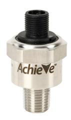
AchieVe pressure transmitter, 0 to 60 psig range, +/- 1% accuracy, stainless steel sensing element, 4-20 mA analog output, 1/4in male NPT process connection, 9-32 VDC operating voltage, 4-pin M12 quick-disconnect.
