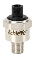
AchieVe pressure transmitter, 0 to 30 psig range, +/-1% accuracy, stainless steel sensing element, 4-20 mA analog output, 1/4in male NPT process connection, 9 to 32 VDC operating voltage, 4-pin M12 quick-disconnect.
