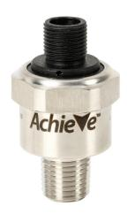
AchieVe pressure transmitter, 0 to 15 psig range, +/- 1% accuracy, stainless steel sensing element, 4-20 mA analog output, 1/4in male NPT process connection, 9-32 VDC operating voltage, 4-pin M12 quick-disconnect.
