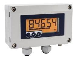
ProSense digital panel meter, field mount, 17mm 5-digit black LCD, bar graph LCD, backlight, analog input, loop powered, hazardous location rated.
