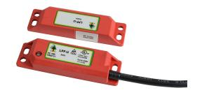
IDEM safety switch set, non-contact uniquely coded RFID, (2) N.C. safety output(s), (1) N.O. monitoring output(s), plastic housing, 88 x 25mm, 8-pin M12 quick-disconnect, 9.8in/250mm cable length.
