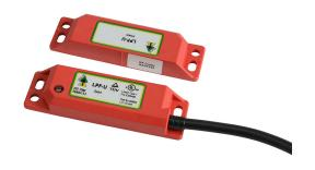
IDEM safety switch set, non-contact uniquely coded RFID, (2) N.C. safety output(s), (1) N.O. monitoring output(s), plastic housing, 88 x 25mm, pigtail, 32.8ft/10m cable length.
