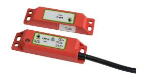
IDEM safety switch set, non-contact uniquely coded RFID, (2) N.C. safety output(s), (1) N.O. monitoring output(s), plastic housing, 88 x 25mm, pigtail, 16.4ft/5m cable length.
