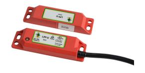
IDEM safety switch set, non-contact uniquely coded RFID, (2) N.C. safety output(s), (1) N.O. monitoring output(s), plastic housing, 88 x 25mm, pigtail, 6.5ft/2m cable length.
