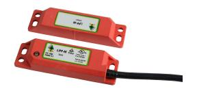
IDEM safety switch set, non-contact master coded RFID, (2) N.C. safety output(s), (1) N.O. monitoring output(s), plastic housing, 88 x 25mm, pigtail, 32.8ft/10m cable length.
