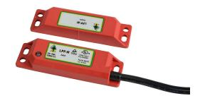
IDEM safety switch set, non-contact master coded RFID, (2) N.C. safety output(s), (1) N.O. monitoring output(s), plastic housing, 88 x 25mm, pigtail, 16.4ft/5m cable length.
