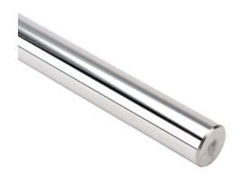
SureMotion linear precision ground shaft, 1060 steel, RC60-65, 10RMS, 0.7495in diameter, 24in length. For use with 3/4in SureMotion bearings.
