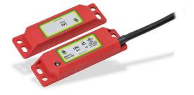
IDEM safety switch set, non-contact coded magnetic, (2) N.C. safety output(s), (1) N.O. monitoring output(s), plastic housing, 88 x 25mm, pigtail, 32.8ft/10m cable length.
