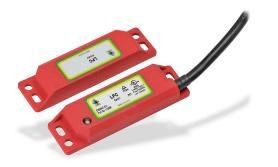
IDEM safety switch set, non-contact coded magnetic, (2) N.C. safety output(s), (1) N.O. monitoring output(s), plastic housing, 88 x 25mm, pigtail, 16.4ft/5m cable length.
