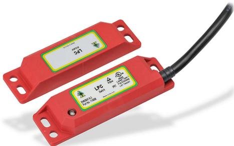
IDEM safety switch set, non-contact coded magnetic, (2) N.C. safety output(s), (1) N.O. monitoring output(s), plastic housing, 88 x 25mm, pigtail, 16.4ft/5m cable length.
