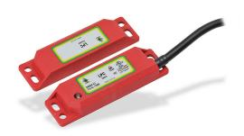
IDEM safety switch set, non-contact coded magnetic, (2) N.C. safety output(s), (1) N.O. monitoring output(s), plastic housing, 88 x 25mm, pigtail, 6.5ft/2m cable length.
