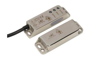
IDEM Z-Range safety switch set, non-contact uniquely coded RFID, (2) OSSD safety output(s), (1) status monitoring output(s), 316 stainless steel housing, 88 x 25mm, 8-pin M12 quick-disconnect, 9.8in/250mm cable length.
