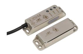
IDEM Z-Range safety switch set, non-contact uniquely coded RFID, (2) OSSD safety output(s), (1) status monitoring output(s), 316 stainless steel housing, 88 x 25mm, pigtail, 32.8ft/10m cable length.
