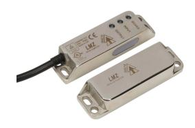
IDEM Z-Range safety switch set, non-contact uniquely coded RFID, (2) OSSD safety output(s), (1) status monitoring output(s), 316 stainless steel housing, 88 x 25mm, pigtail, 16.4ft/5m cable length.
