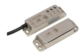
IDEM Z-Range safety switch set, non-contact master coded RFID, (2) OSSD safety output(s), (1) status monitoring output(s), 316 stainless steel housing, 88 x 25mm, 8-pin M12 quick-disconnect, 9.8in/250mm cable length.
