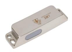
IDEM Z-Range safety switch actuator, replacement, non-contact master coded RFID, 316 stainless steel housing, 88 x 25mm.
