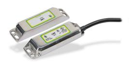
IDEM safety switch set, non-contact magnetic, (2) N.C. safety output(s), (1) N.O. monitoring output(s), 316 stainless steel housing, 88 x 25mm, pigtail, 32.8ft/10m cable length.
