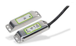
IDEM safety switch set, non-contact magnetic, (2) N.C. safety output(s), (1) N.O. monitoring output(s), 316 stainless steel housing, 88 x 25mm, pigtail, 16.4ft/5m cable length.
