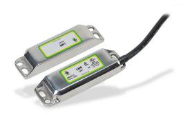
IDEM safety switch set, non-contact magnetic, (2) N.C. safety output(s), (1) N.O. monitoring output(s), 316 stainless steel housing, 88 x 25mm, pigtail, 6.5ft/2m cable length.
