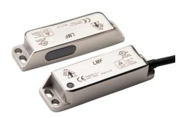
IDEM safety switch set, non-contact uniquely coded RFID, (2) N.C. safety output(s), (1) N.O. monitoring output(s), 316 stainless steel housing, 25 x 88mm, 8-pin M12 quick-disconnect, 9.8in/250mm cable length.
