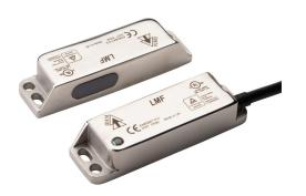
IDEM safety switch set, non-contact uniquely coded RFID, (2) N.C. safety output(s), (1) N.O. monitoring output(s), 316 stainless steel housing, 25 x 88mm, pigtail, 32.8ft/10m cable length.
