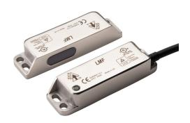
IDEM safety switch set, non-contact master coded RFID, (2) N.C. safety output(s), (1) N.O. monitoring output(s), 316 stainless steel housing, 25 x 88mm, 8-pin M12 quick-disconnect, 9.8in/250mm cable length.
