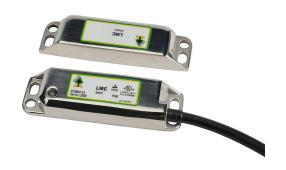
IDEM safety switch set, non-contact coded magnetic, (2) N.C. safety output(s), (1) N.O. monitoring output(s), 316 stainless steel housing, 88 x 25mm, 8-pin M12 quick-disconnect, 9.8in/250mm cable length.
