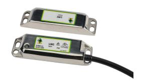
IDEM safety switch set, non-contact coded magnetic, (2) N.C. safety output(s), (1) N.O. monitoring output(s), 316 stainless steel housing, 88 x 25mm, 8-pin M12 quick-disconnect, 9.8in/250mm cable length.
