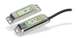
IDEM safety switch set, non-contact coded magnetic, (2) N.C. safety output(s), (1) N.O. monitoring output(s), 316 stainless steel housing, 88 x 25mm, pigtail, 16.4ft/5m cable length.
