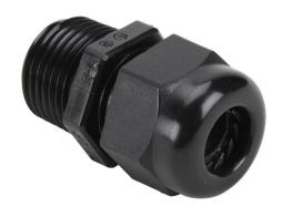
Cable gland, 1/2in male NPT thread type, nylon, accepts 0.180 to 0.400in (4.6 to 10.2mm) diameter cable. Buna N sealing gland included.
