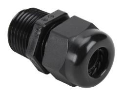
Cable gland, 1/2in male NPT thread type, nylon, accepts 0.180 to 0.400in (4.6 to 10.2mm) diameter cable. Buna N sealing gland included.
