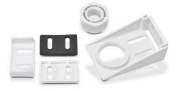
Flowline side mount bracket, polypropylene, 2in female NPT. For use with Flowline DL14, DL24, DS14, DL10, DX10, LU27, LU77 and LU80 series ultrasonic level sensors. 2in male NPT to 1in female NPT reducer bushing (PVC) included.
