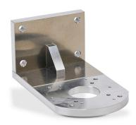
Koyo right angle bracket, metal. For use with Koyo TRDA-20 series encoders. Mounting hardware included. Requires TRDA-20SND or TRDA-25SND replacement mounting flange and (4) customersupplied #6-32 UNC x 1/2in fasteners.
