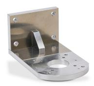
Koyo right angle bracket. For use with Koyo TRDA-20 series encoders. Mounting hardware included. Requires TRDA-20SND or TRDA-25SND replacement mounting flange and (4) customer-supplied #6-32 UNC x 1/2in fasteners.
