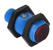
Contrinex photoelectric sensor, tubular, threaded, ABS plastic housing, through-beam receiver, 0-30m sensing distance, 10-30 VDC operating voltage, complementary light-on/dark-on, PNP, 4-wire, 4-pin M12 quick-disconnect.
