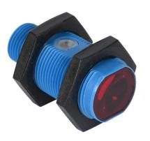
Contrinex photoelectric sensor, tubular, threaded, ABS plastic housing, through-beam emitter, visible red, 0-30m sensing distance, 10-30 VDC operating voltage, 3-wire, 4-pin M12 quickdisconnect.
